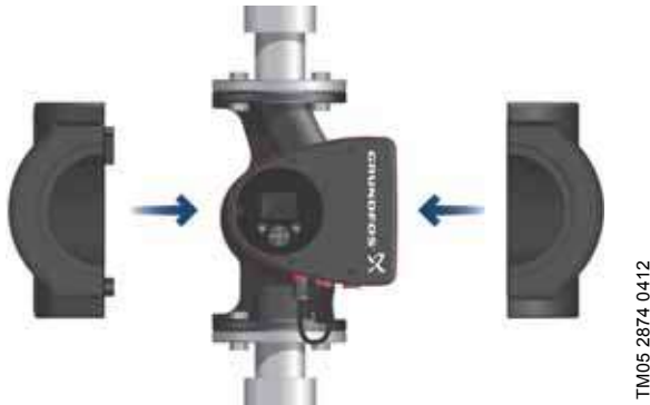
Fig. 44 Fitting the insulating shells to a MAGNA3 pump
